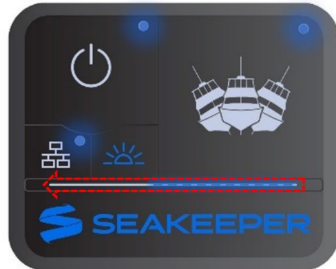
Figure 7B: Spool bar LEDs will strobe right to left for DHCP OFF.
