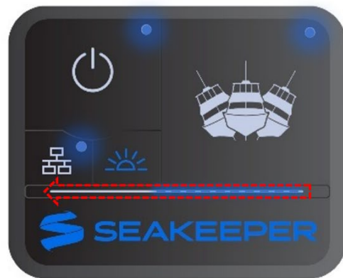
Figure 13B: Spool bar LEDs will strobe right to left for DHCP OFF.
