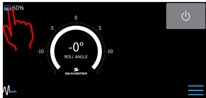
Figure 25: Home screen with SoC monitoring
