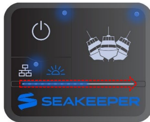
Figure 11B: Spool bar LEDs will strobe left to right for DHCP ON.
