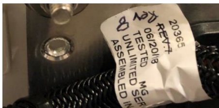
Seakeeper 2 harness should be Rev. 8 or later.
