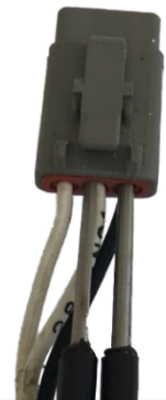
Angle sensor harness connector with back probes installed
