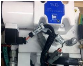
Seakeeper 16 Hirschmann plug shown on proportional valve
