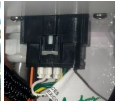
Molex Connector of an AC-powered Seakeeper shown with white locking tab fully inserted
