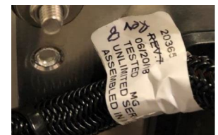
Harness revision tag for Seakeeper 2
