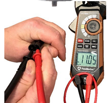
Meter in this photo is displaying 11.05 KΩ.
