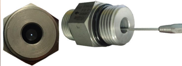
Technician inspecting and cleaning an adapter-type check valve.
