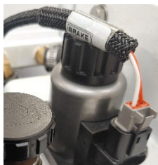
An example of brake solenoid assembly
