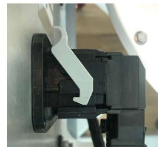
GCM connector fully inserted and locked
