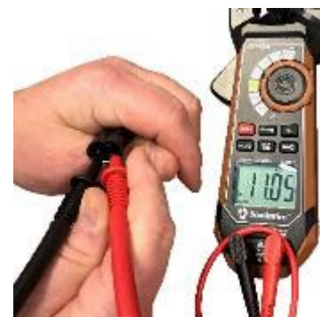
Meter in this photo is displaying 11.05 KΩ.
