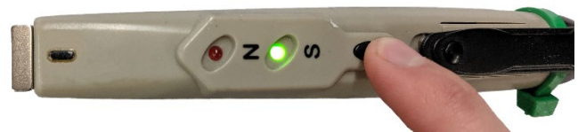
An example of pole detection device in operation with magnet.
