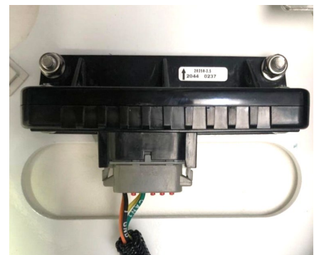
Seakeeper 18/16 IMU shown inside rear panel
