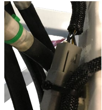
Photo showing location of Guide Band connector inside foundation near guide band bracket and below manifold.
