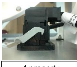
A properly connected GCM 70-pin connector
