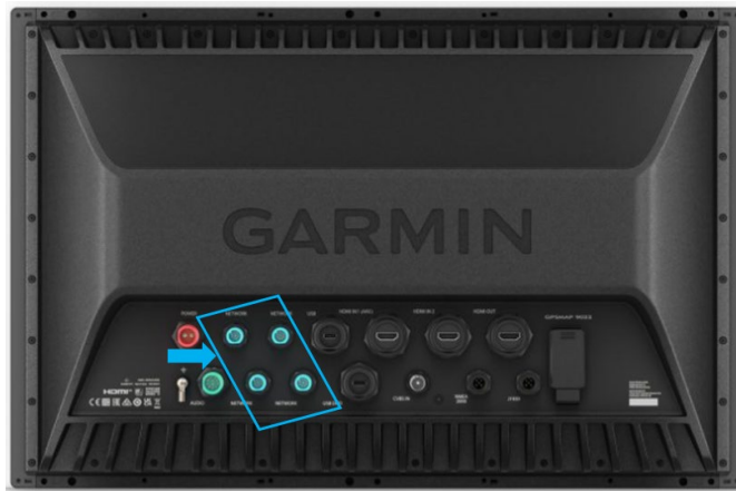
Figure 8: Connect Seakeeper Cable P/N 20617 to a "Network" Port on the Back of the 9000 Series MFD
