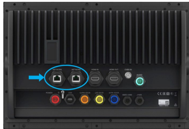
Figure 6: Connect Cable 20373 to a "Network" Port on the Back of the MFD
