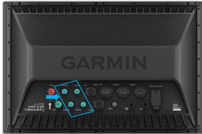
Figure 7: Connect Seakeeper Cable P/N 20617 to a "Network" Port on the Back of the 9000 Series MFD
