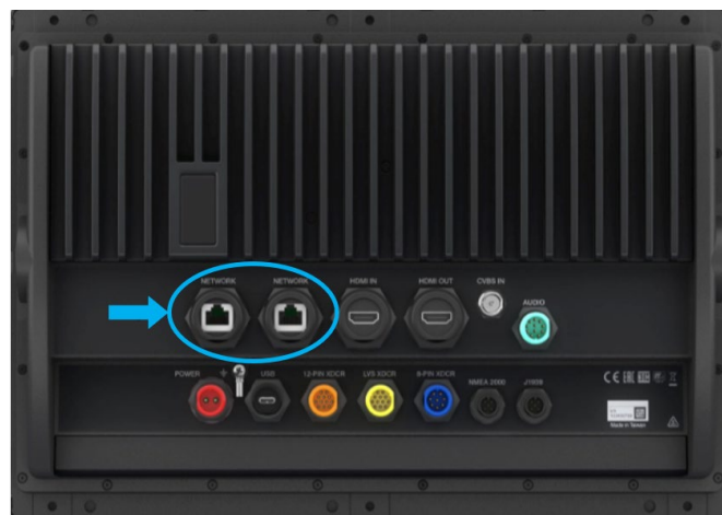
Figure 2: Garmin RJ45 Network ports
