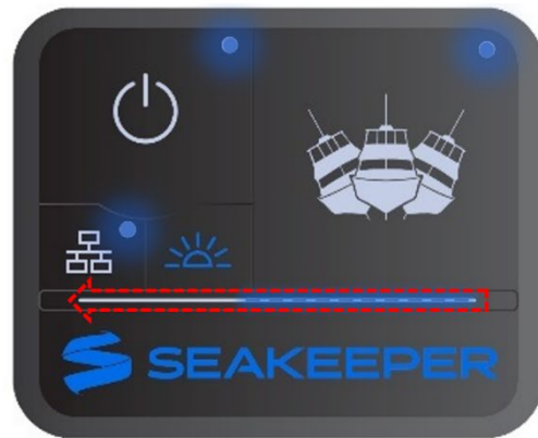
SPOOL BAR LEDs WILL STROBE FROM RIGHT TO LEFT. ROUND LEDs WILL FLASH
