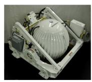
Seakeeper M26000 gyro designed to reduce roll by 80 percent on vessels up to 100 feet long
