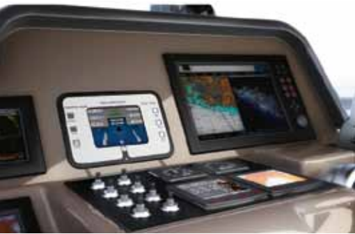
▲ CMC fin stabiliser panel control
